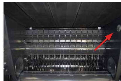
Moisture sensor located inside the bale chamber.
