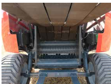
A combination of 5 belts and front rollers provides dense bales with a soft core and a easy bale start.
