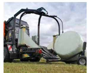
Bale turner option. During transport the kit is automatically pivoted into a safe position on the wrapping unit.
