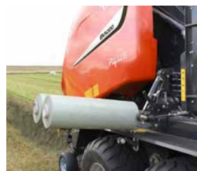
Twin cassettes for 10 spare film rolls operated hydraulically.
