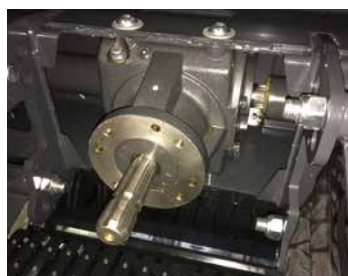
The split drive gearbox on rotor intake models provides even power distribution reducing wear.
